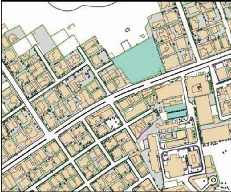
Figure 16: Example of 1:1,000 base map with some of the over hundred features of the geo-database.
