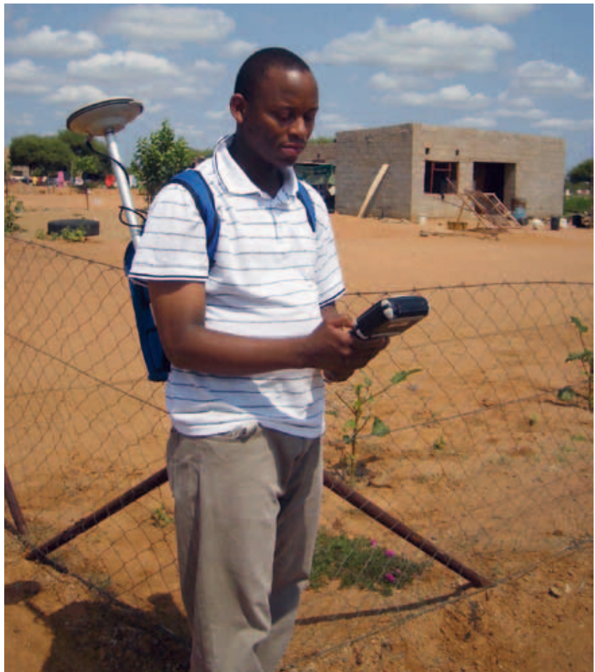
GPS technology can help survey plots to sub-metre accuracy
